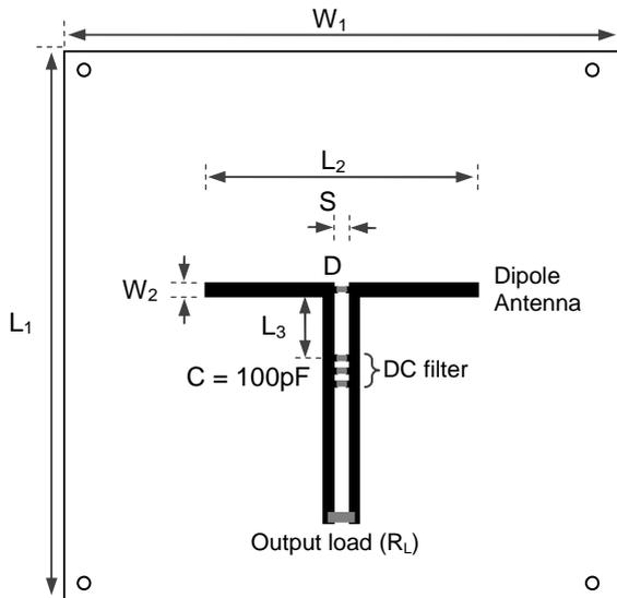
Figure 1. Layout of the single rectenna.  $L_1 = 100$ ,  $L_2 = 45$ ,  $L_3 = 12$ ,  $W_1 = 100$ ,  $W_2 = 4$ ,  $S = 3$  (all dimensions are in mm)
