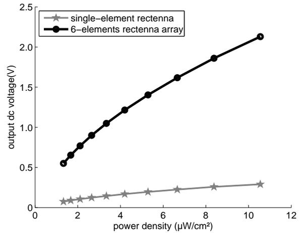
Figure 3. Measured output dc voltage versus power density
