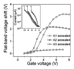
FIG. 4. Flat-band voltage shift ( $\Delta V_{FB}$ ) as a function of the gate voltage round sweep for 7-nm-thick oxide layers implanted with  $2\times 10^{16}$  Si/cm² at 1 keV and subsequently annealed following the A1, A2, or A3 treatment. Inset: Magnitude of the dark gate current under accumulation conditions as a function of negative ramped gate voltage (1 V/s).
