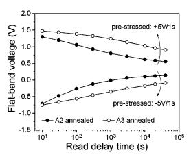
FIG. 5. Data retention characteristics of 7-nm-thick oxide layers implanted with  $2\times10^{16}~\text{Si/cm}^2$  at 1 keV and subsequently A2 or A3 annealed. The magnitude of the applied gate voltage stress was +5~V or -5~V for 1 s.
