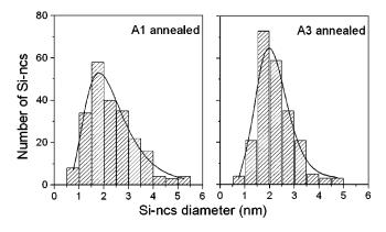
FIG. 2. Nanocrystal size distribution measured from plane-view TEM images of 7-nm-thick  ${\rm SiO_2}$  annealed according to the A1 or A3 treatment. The number-average size (mean size) is around of 2 nm for both samples.
