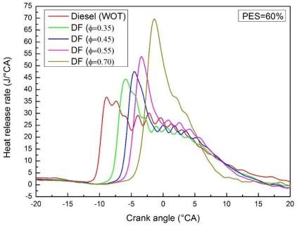
Fig.4. Heat release rate (HRR) with crank angle for different  $\phi$ .
