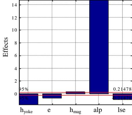
Figure 11. Factor influences on the noise amplitude
