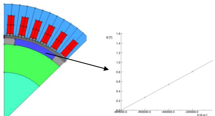
Figure 1. 1/8 of synchronous machine with magnet characteristic
