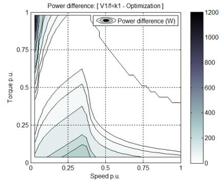
Fig. 15. Power map comparison: [Optimization map –  $V_1/f=k_i$  map]
