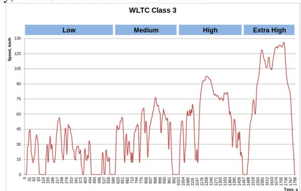
Fig. 16. WLTC driving cycle for class 3 vehicles
