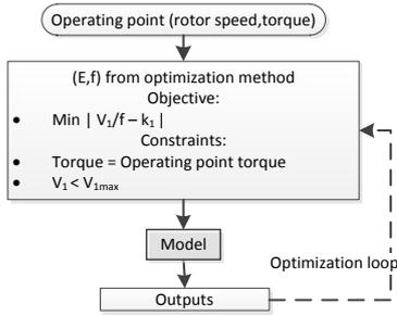
Fig. 4. Optimization method to get  $V_1/f=k_1$
