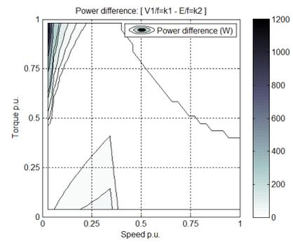
Fig. 14. Power map comparison: [ $E/f=k_2$  map –  $V_1/f=k_i$  map]
