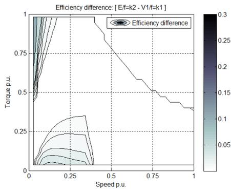
Fig. 11. Efficiency map comparison: [ $E/f=k_2$  map –  $V_1/f=k_i$  map]
