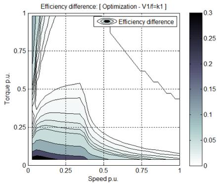
Fig. 12. Efficiency map comparison: [Optimization map –  $V_1/f=k_i$  map]
