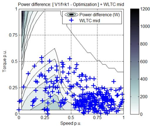
Fig. 18. Power comparison + WLTC mid operating points
