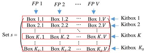
In this case, the considered cycle time is that of the whole set  $s$  preparation. The assessed cycle time should be then equal to the time needed to prepare one kit or one FP multiplied by  $V$  the number of FPs in each set  $s$ .
