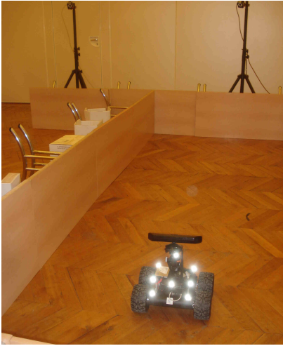
Fig. 3: Wifibot robot in its testing arena, surrounded by Optitrack cameras
