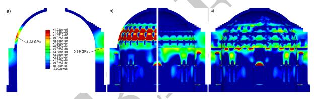
Figure 10: Hoop stresses due to self-weight with and without stepped rings: a) 2D axisymmetric, b) 3D model, and c) 3D model at the end of the shrinkage calculations,  $(\varepsilon_v/\alpha)_5 = 4.55$  K (cracks are not displayed).
