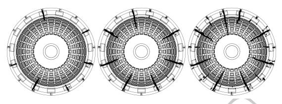
Figure 7: Progressive cracking of the dome due to an incrementally applied thermal load of  $(\varepsilon_v/\alpha)_5 = 4.55$  K, during step 2) (plan view).
