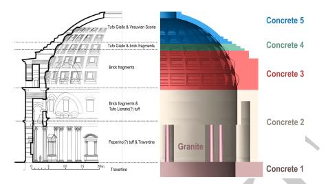
Figure 3: Materials composing the *Rotonda* as in [Lancaster, 2005] (left) and in Table 1.
