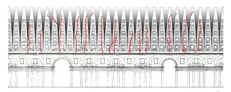
Figure 2: Meridional cracks in the *Rotonda's* dome (after [Terenzio, 1934]).
