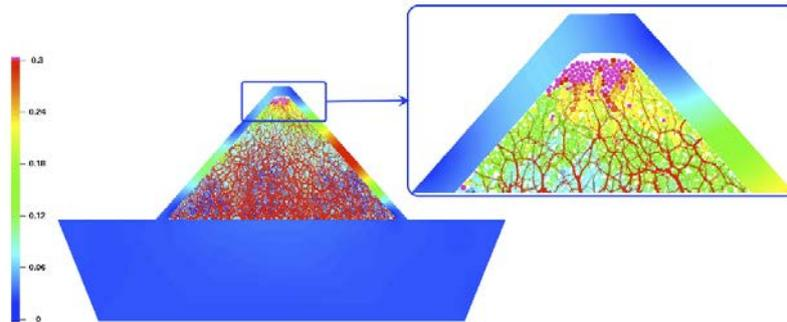
Fig. 11 – Rearrangement at top of dam after seism
