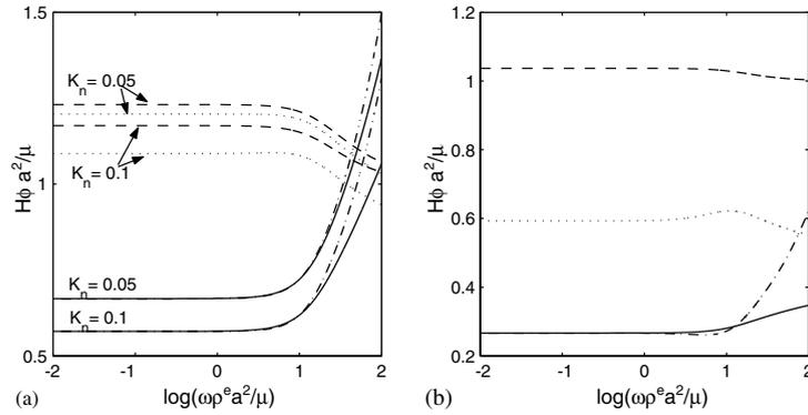
Fig. 3. Variations of  $H_{\text{eff}}$  (real part in plain line and imaginary part in dashed line) and  $H_{\text{app}}$  (real part in dash-dot line and imaginary part in dot line) with respect to the dimensionless pulsation: (a) for distinct low values of the Knudsen number; (b) for  $K_n = 0.5$ .
