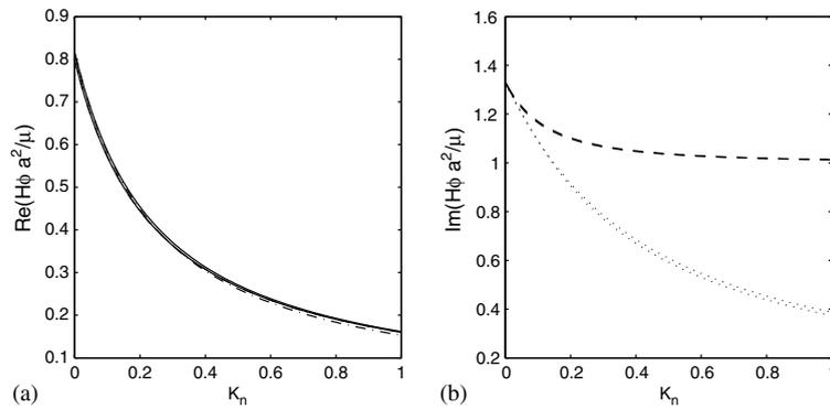
Fig. 4. (a) Variations of the real part of  $H_{\text{eff}}$  (in plain line) and of  $H_{\text{app}}$  (in dash-dot line) with respect to the Knudsen number for two values of the pulsation ( $w^* = 0.5$  and  $w^* = 5$ ). (b) Variations of the imaginary part of  $H_{\text{eff}}$  (in dashed line) and  $H_{\text{app}}$  (in dot line) with respect to the Knudsen number for the same two values of the pulsation.
