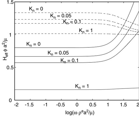
Fig. 2. Variations of  $H_{\text{eff}} = H_1 + iH_2$  with respect to the dimensionless pulsation for distinct values of the Knudsen number. Plain line:  $0.1H_1$  (dissipative term); dashed line:  $\omega^{-1}H_2$  (inertial term).
