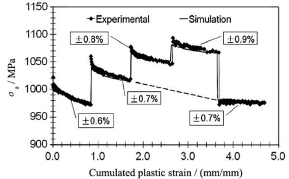
Fig. 4. Experiment-simulation comparison: stress amplitude-cumulated plastic strain for a type two test on sample 45.5HRC tested at 573 K.
