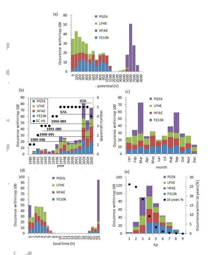
**Figure 6** – Number of occurrences within the top 100 events, for each class of event (color-coded), as a function of (a) LANL spacecraft potential, (b) year, (c) month, (d) local time and (e) Kp index selected out of the 16 years of LANL data. The number of spacecraft hosting LANL sensors and their lifetime are also presented in (b). The relative occurrence frequency of the Kp index is also plotted in (e).
