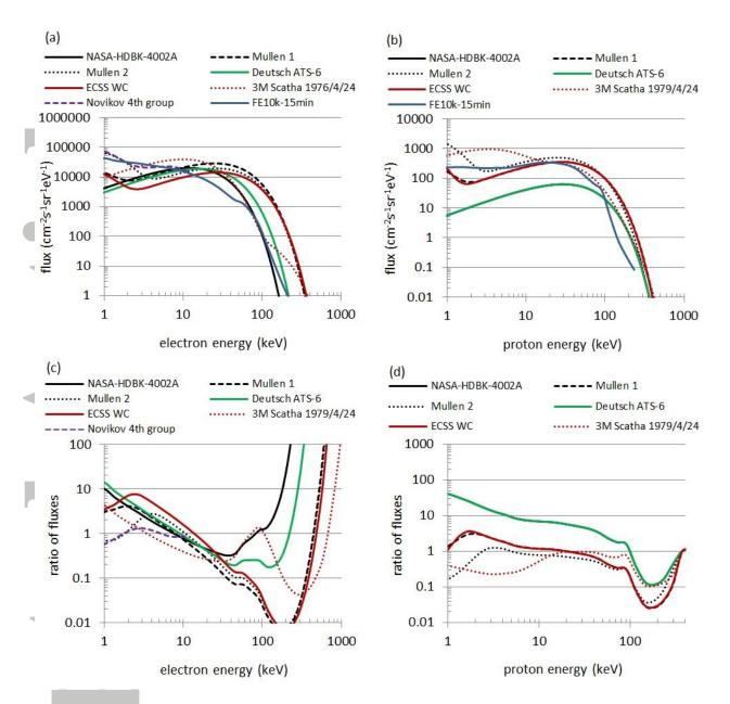
**Figure 12** – Worst-case spectra from the literature and the FE10k-15min worst-case, for (a) electrons and (b) protons. Ratio of the FE10k over each of the guidelines worst-case, for (c) electrons and (d) protons.
