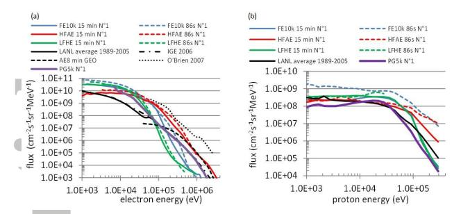
**Figure 11** - (a) Electron and (b) proton differential fluxes during the worst case FE10k, HFAE, LFHE and PG5k events, compared to the average LANL flux, to the AE8 and IGE 2006 specifications and to the worst 1 hour interval reconstructed spectrum from *O'Brien et al.* [2007] concerning graph (a).
