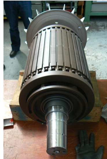
Fig. 11. New rotor of the industrial 250 kW motor.
