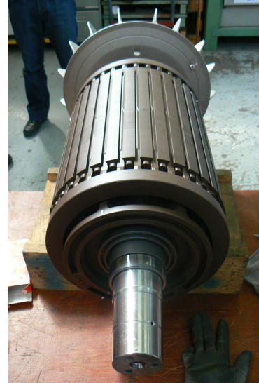
Fig. 11. New rotor of the industrial 250 kW motor.
