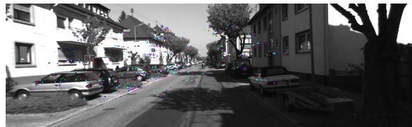
Fig. 4. Example of reprojection errors of the 3D points after BA, each color refers to the reprojection errors on a camera of the sliding window (5 cameras)
