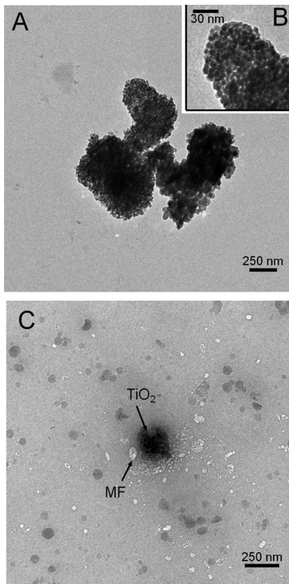
**Fig 1.** TEM images of (A) 0.5 mg/mL TiO<sub>2</sub> NPs alone; (B): enlarged view of the cluster; (C) 0.5 mg/mL TiO<sub>2</sub> NPs with membrane fraction (MF) (25 μg/mL *cyt b558*) and 50 μg/mL aggregated trimera;. (The black bar gives the scale: 250 nm for Fig 1A and 1C and 30 nm for Fig 1B). The samples are dried (see [materials and methods](#)).
