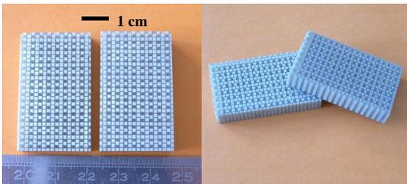
Fig. 4. Pictures of fabricated super-cell 1-3 piezocomposites.
