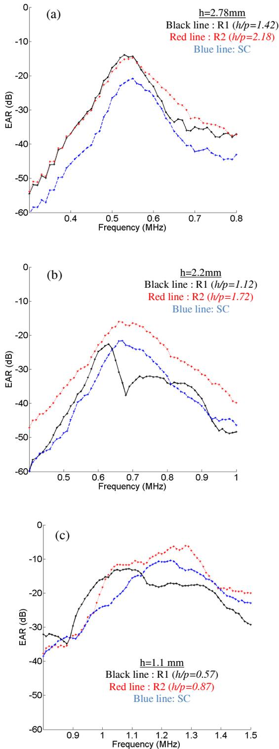
Fig. 5. Experimental electroacoustic responses (EAR) as a function of frequency for the three fabricated 1-3 piezocomposites (R1: regular with 2 mm pitch value, R2: regular with 1.33 pitch value, SC: super-cell): for a thickness of (a) 2.78 mm, (b) 2.2 mm and (c) 1.1 mm.
