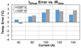
Fig. 15: Temperature measurement via  $I_{\text{GPeak}}$ : error vs. gate pad temperature.
