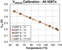
Fig. 12:  $V_{\text{CE(low)}}$  vs. Temperature from calibration data for IGBT A and B
