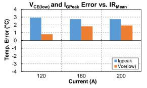
Fig. 26:  $I_{\text{GPeak}}$  and  $V_{\text{CE(low)}}$  on 2 paralleled IGBTs (IGBT A): error vs. cumulative mean surface temperature.
