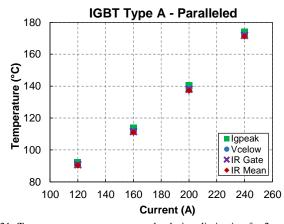
Fig. 21: Temperature measurement results during dissipation for 2 paralleled IGBTs (IGBT A) from 120A-240A.
