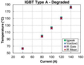
Fig. 18: Temperature measurement results during dissipation on IGBT A with bondwires removed.
