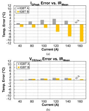
Fig. 13: Measurement error vs. mean surface temperature for (a)  $I_{\text{GPeak}}$  and (b)  $V_{\text{CE(low)}}.$
