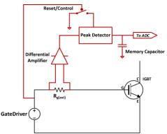
Fig. 1. Peak Detector Schematic to detect peak voltage over the external
