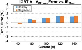
Fig. 20: Temperature measurement via  $V_{\text{CE(low)}}$ : error vs. mean surface temperature in healthy and degraded condition
