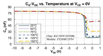
Fig. 8. C<sub>G</sub>-V<sub>GE</sub> vs. temperature profile for IGBT A (Infineon FS200R12PT4)
