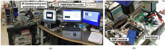
Fig. 5. (a) Panoramic view of test bench (b) Close up of power module, IR Camera, and gate driver with peak detector measurement circuit [11]
