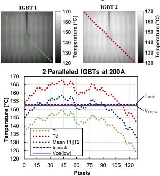
Fig. 25: Temperature profile of 2 paralleled IGBTs (IGBT A) with 200A heating current. Temperature is plotted along diagonal lines.
