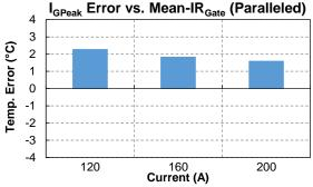
Fig. 24: I<sub>GPeak</sub> on 2 paralleled IGBTs (IGBT A) with a temperature disequilibrium: error vs. cumulative mean of gate pad temperature.
