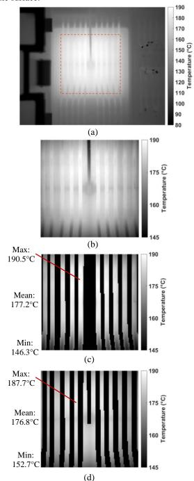
Fig. 9. Processing of IR images to extract the junction temperature:
