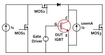
Fig. 6. Test Bench Schematic
