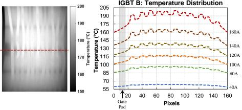
Fig. 16: Temperature profile across IGBT B from 40A to 160A. Temperature is plotted along the dotted line
