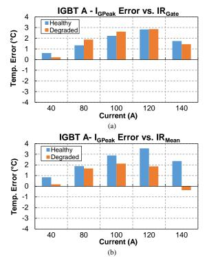
Fig. 19: Temperature measurement via  $I_{\text{GPeak}}$  in degraded and healthy conditions: (a) Error vs. gate pad temperature. (b) Error vs. mean surface temperature.
