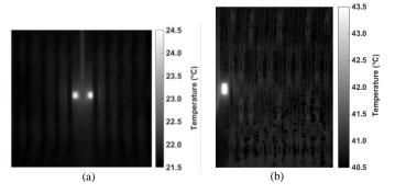
Fig. 10. Self-heating of R<sub>Gint</sub>: (a) IGBT A. (b) IGBT B.
