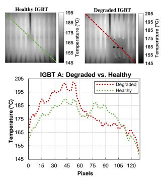
Fig. 17: Comparison of IGBT A temperature profile at 140A before and after bondwire removal. Temperature is displayed along diagonal lines
