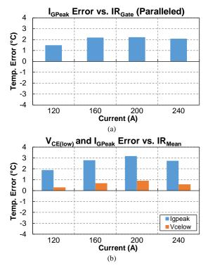
Fig. 22: Temperature measurement error for 2 paralleled IGBTs (IGBT A), (a)  $I_{\text{GPeak}}$  error vs. gate pad temperature. (b)  $I_{\text{GPeak}}$  and  $V_{\text{CE(low)}}$  errors vs. mean surface temperature.
