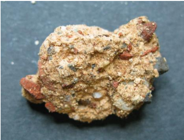
Figure 5 – Sample C2, mortar with cocchiopesto
