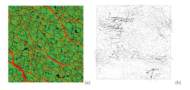
FIG. 3. (a) A map of normal forces in a polydisperse packing of disks. Line thickness is proportional to normal force; (b) A map of nonaffine particle displacements in a sheared packing of disks.
