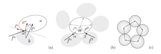
FIG. 2. (a) The contact geometry; (b) First-shell particle environment with angular exclusions; (c) A loop of touching particles.
