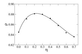
FIG. 6. The packing fraction of an assembly of nonconvex agregates each composed of three overlapping disks as a function of the degree of nonconvexity  $\eta$ .
