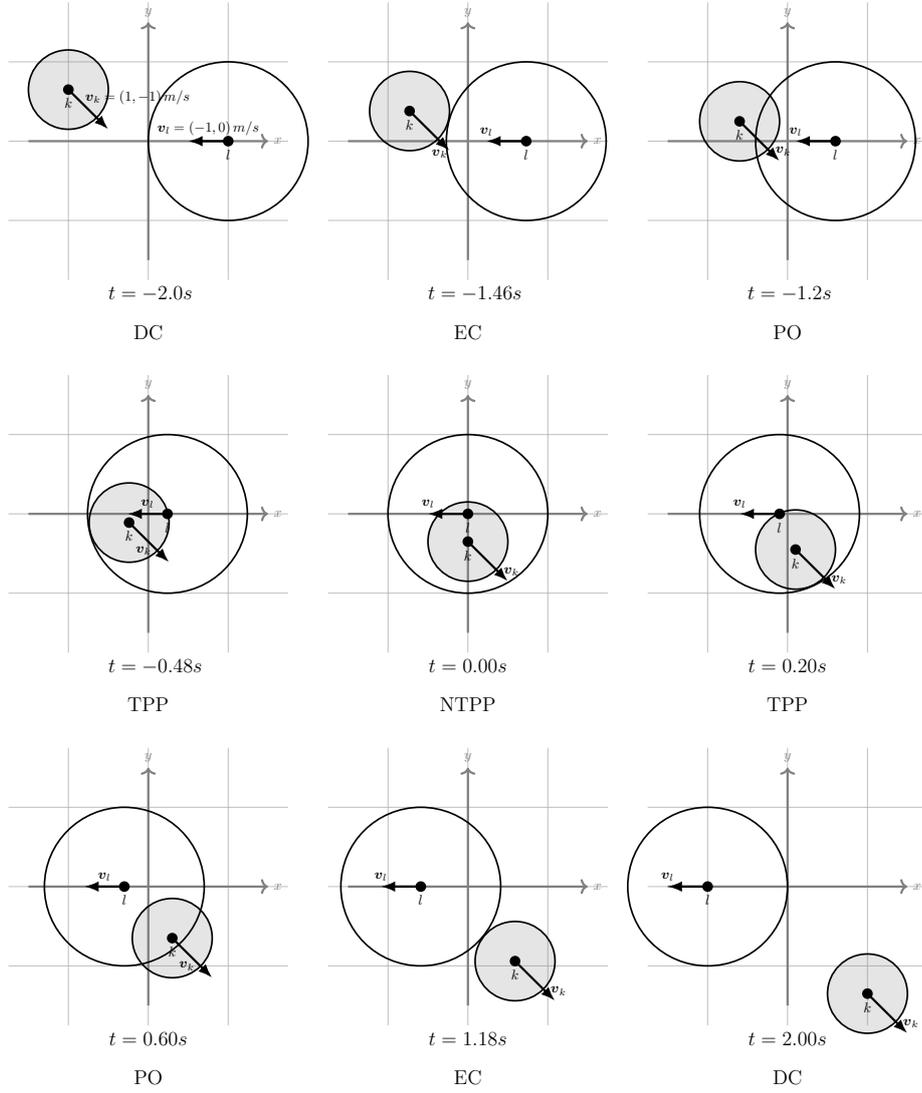
**Fig. 2. A RCC story with nine qualitative relations.** Two circular entities  $k$  (radius =  $1m$ ) and  $l$  (radius  $2m$ ) moving in uniform motion with velocities  $v_k = (1, -1) m/s$  and  $v_l = (-1, 0) m/s$ . They depict the Temporal Sequence of Relations (DC, EC, PO, TPP, NTPP, TPP, PO, EC, DC) in the qualitative representation RCC (Fig. 3). The snapshots correspond to different increasing times.
