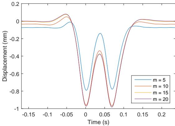
**Fig. 4** Numerical results with different numbers of iterations for the cubic-nonlinear foundation
