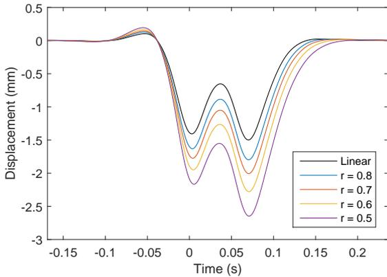
**Fig. 8** Effect of the nonlinear parameter of the bilinear foundation on the block displacement
