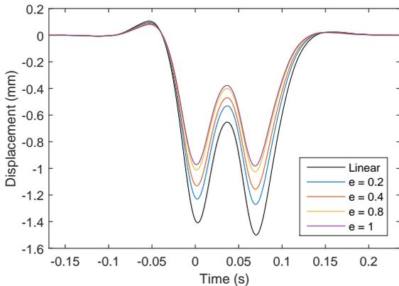
**Fig. 5** Effect of the nonlinear parameter of the cubic-nonlinear foundation on the block displacement
