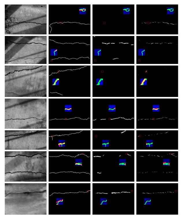
**Fig. 9** Examples of the results obtained on the blurred images: the proposed approach using NFA criterion (first column), the approach using FFA measure<sup>22</sup> (second column), and the percolation approach<sup>4</sup> (third column). Red squares highlight some areas which were magnified for a detailed visualization (the color code is specified in the text).
