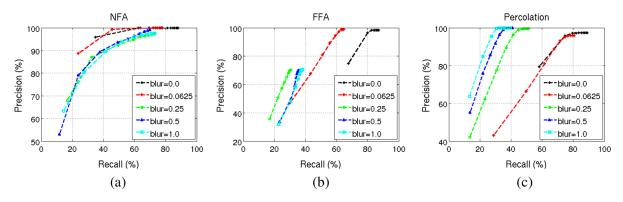
**Fig. 11** Validation of the proposed approach and comparison with alternatives in terms of the Precision and Recall versus the scale of the analysis, and for varying levels of blur: (a) performance of the proposed method (NFA), (b) performance of "FFA," and (c) performance of "percolation."
