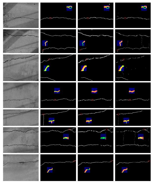
**Fig. 8** Examples of the results obtained on the original images: the original images (first column), the proposed approach using NFA criterion (second column), the approach using FFA measure<sup>22</sup> (third column), and the percolation approach<sup>4</sup> (fourth column). Red squares highlight some areas which were magnified for a detailed visualization (the color code is specified in the text).
