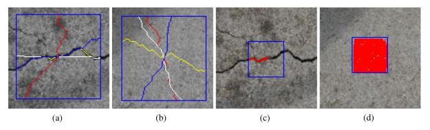
Fig. 1 Behavior of (a, b) free-form anisotropy (FFA) and (c, d) percolation local analysis methods for crack pixels and normal areas, respectively.
