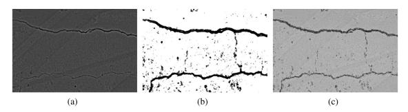
**Fig. 4** Derivation of the image  $Y_{\tilde{l}}$  in (c), used for crack detection as a linear combination of background subtraction in (a) with  $\tilde{l} = l - f_{G(\sigma)} * \phi(l)$  [*l* being shown in Fig. 3(a)], and ratio image  $r_{\tilde{l}}$  [Eq. (5)] shown in (b), here with  $\alpha = 0.5$ .
