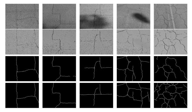
Fig. 12 Examples of the results obtained on the crack dataset<sup>3</sup> with the original images shown on the first line, the composite image shown on the second line, the proposed approach results shown on the third line, and the ground truth images shown on the fourth line.
