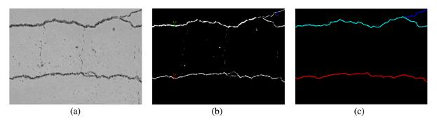
**Fig. 7** Example of intermediate results provided by Algorithm 3: (a) gray level image  $Y_{\bar{i}}$ , (b)  $I_{\hat{D}_s}$  dilation with the different seeds (highlighted in color) selected iteratively, (c) subparts of the crack reconstructed iteratively: first iteration: red subpart obtained from red seed  $s_1$  (bottom left), second iteration: cyan subpart obtained from green seed  $s_2$  (top left), third iteration: both cyan and blue subparts obtained from blue seed  $s_3$  (top right).
