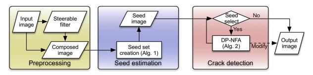
**Fig. 2** A comprehensive flowchart of the different processing steps. The preprocessing part is introduced in Sec. 3.1, and Algorithms 1 and 2 are detailed in Sec. 3.5. Algorithm 3, also presented in Sec. 3.5, corresponds to the entire flowchart.
