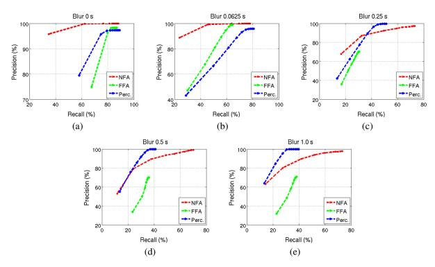
**Fig. 10** Validation of the proposed approach (NFA) and comparison with alternatives ("percolation" and "FFA") in terms of the Precision and Recall versus the scale of the analysis. The simulated exposure time T (in s) varies among the illustrations above, (a) case of original images (T = 0), (b) blur with T = 0.0625, (c) blur with T = 0.25, (d) blur with T = 0.5, and (e) blur with T = 1.
