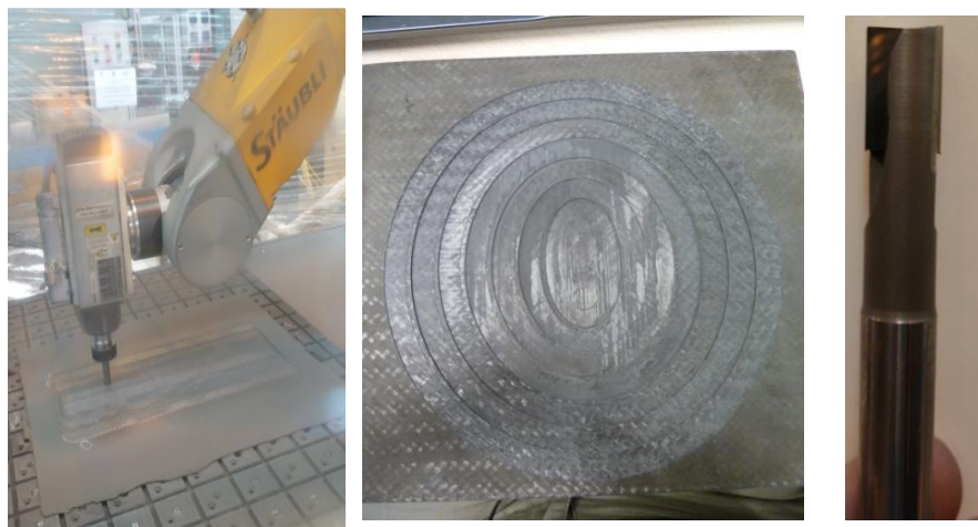
Fig 8 Stepped lab composite part produced by the robot
