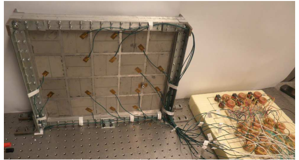
Figure 12: Clamped aluminum plate covered with piezoelectric patches connected to the multi-resonant network.
