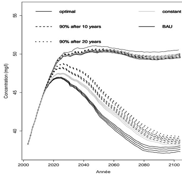
Figure 6: Nitrate concentration path related to scenarios differing in tax path and livestock adjustment, regarding the two targets (long-term value of 50 and 38  $mgNO_3/l$  in the aquifer), when the tax path is optimal (solid black), constant (solid gray), reaches 90% of the steady state tax exponentially in 20 years (dashed) and in 10 years (dotted), and when the amplitude of livestock adjustment changes from 0 (bottom) to 45% (top) of initial livestock by increments of 15%.
