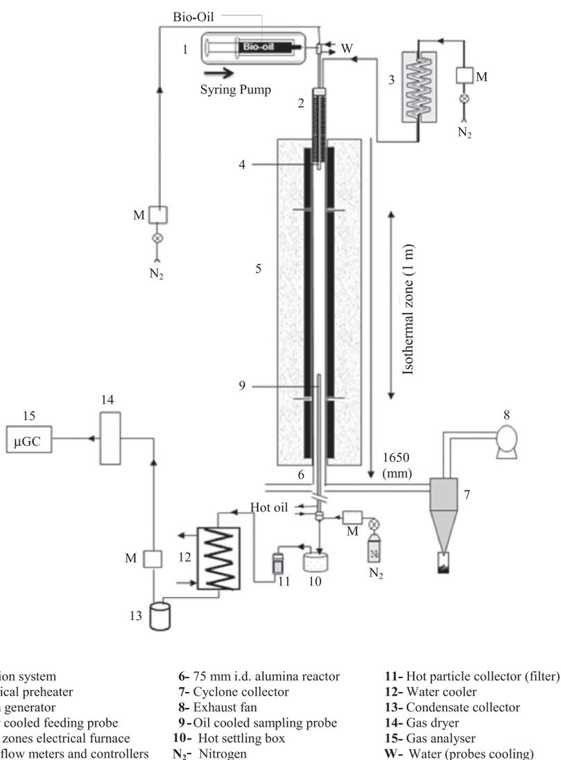
Fig. 2. Entrained Flow Reactor (EFR).
