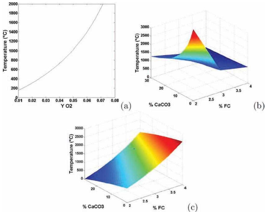
**Figure 11.** Theoretical temperature of the front in the RT mode versus (a) the molar fraction of oxygen in the fed air, and (b) the medium composition in FC and CaCO<sub>3</sub> of the porous medium. (c) Results in RL mode are reminded. The reference conditions for all cases are 3.5% FC, 22.4% CaCO<sub>3</sub>, and 4.5% O<sub>2</sub> in the fed air.
