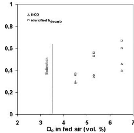
Figure 9. Identified values for the fraction of carbon oxidized to CO and the fraction of CaCO<sub>3</sub> decarbonated.
