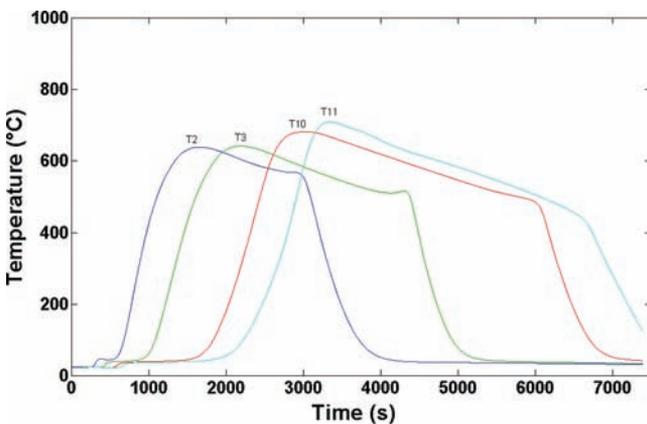
Figure 3. Typical time evolution of the temperature at several locations at the cell axis (T2, T3, T10, and T11). Experiment with  $\text{O}_2 = 5.3 \text{ vol } \%$ , and air superficial velocity =  $0.085 \text{ m s}^{-1}$  at STP.
