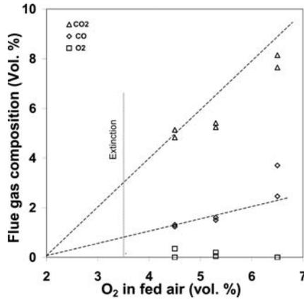
Figure 8. O<sub>2</sub>, CO, and CO<sub>2</sub> concentrations in flue gas versus O<sub>2</sub> concentration in the fed air.
