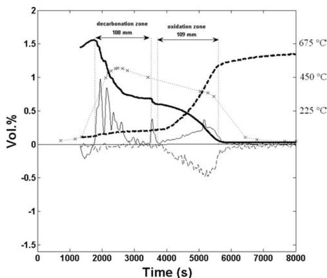
**Figure 10.** Time evolution of the fractions of oxygen (bold dotted line) and carbon dioxide (bold solid line), derivative curves of oxygen (dotted line) and carbon dioxide (solid line) signals, and temperature profile (cross symbols).
