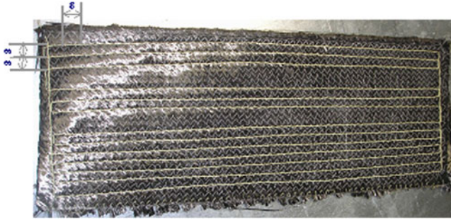
Fig. 3 Stitched preform (assembly of NCF)
