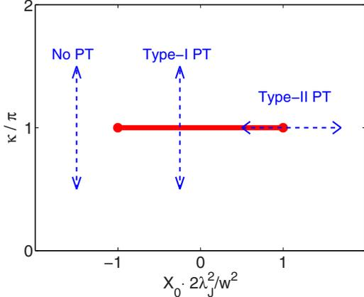
FIG. 8. The  $X_0$ - $\kappa$  diagram showing the line of the type-I phase transition ending with two critical points (red straight curve). The blue dashed curves show the possible trajectories of the Abrikosov vortices corresponding to different type of the phase transitions (PT).
