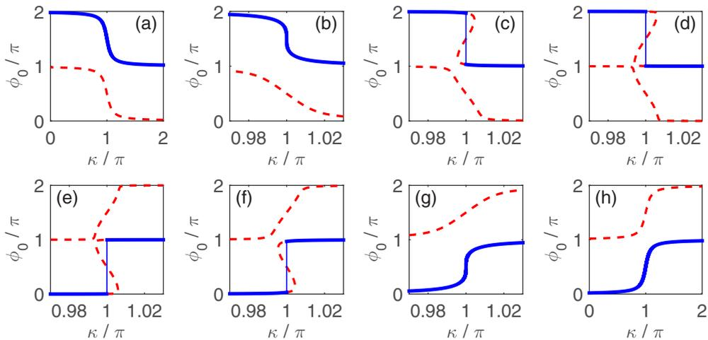
FIG. 7. The dependencies of the ground state phase  $\phi_0$  on the phase jump  $\kappa$  for different values of the vortex position  $X_0$ . The value  $X_0$  is equal to (a)  $-10^{-1}$ ; (b)  $-10^{-2}$ ; (c)  $-10^{-3}$ ; (d)  $-10^{-4}$ ; (e)  $10^{-4}$ ; (f)  $10^{-3}$ ; (g)  $10^{-2}$ ; (h)  $10^{-1}$ . The blue solid lines correspond to the stable branches realizing the minima of the free energy while the red dashed curves show the metastable solutions for  $\phi_0$ .
