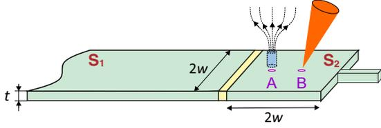
FIG. 9. The sketch of the Josephson junction which enables optical switching of the critical current by the controllable vortex displacement. The  $S_2$  lead has the form of the square of the size  $2w \times 2w$  and contains two artificial defects A and B which can efficiently trap the vortex. The laser beam focused at the nonoccupied pinning center creates an attractive thermal force acting on the vortex and provokes the jump of the vortex from one pinning center to another.
