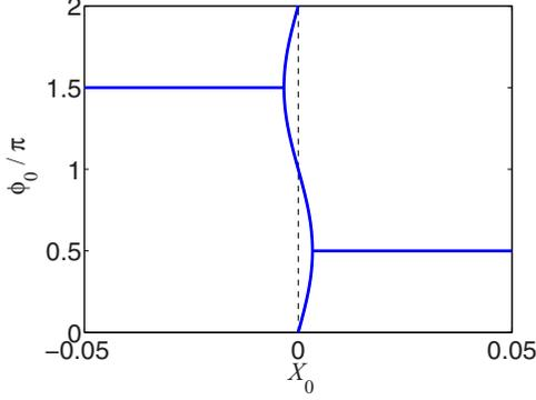
FIG. 5. The dependence of the equilibrium Josephson phase  $\phi_0$  on the vortex position  $X_0$  near the phase transition. The distance between the vortex and the junction is chosen in a way that the phase jump  $\kappa = \pi$ . The junction width is  $w = 0.1\lambda_J$ .
