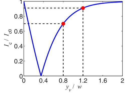
FIG. 12. The dependence of the critical current on the distance  $y_v$  between the vortex and the insulating layer (adopted from Ref. [33]). We take  $x_v = 0$  assuming that the vortex is placed at the central line of the junction. The red points indicate the position of the pinning centers A and B. The critical current is normalized at the value  $I_{c0} = 2j_c w t$ .
