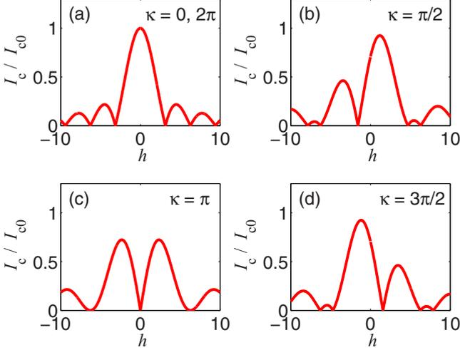
FIG. 4. Asymmetry in the Fraunhofer oscillations of the critical current in the case when the Abrikosov vortex is pinned along the line  $x_0 = 0$  but at different distances  $y_0$ . The Josephson phase jump  $\kappa$  corresponding to  $y_0$  is indicated in each panel.
