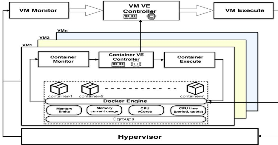
**Figure 1:** Coordinated elastic controllers between VMs and containers
