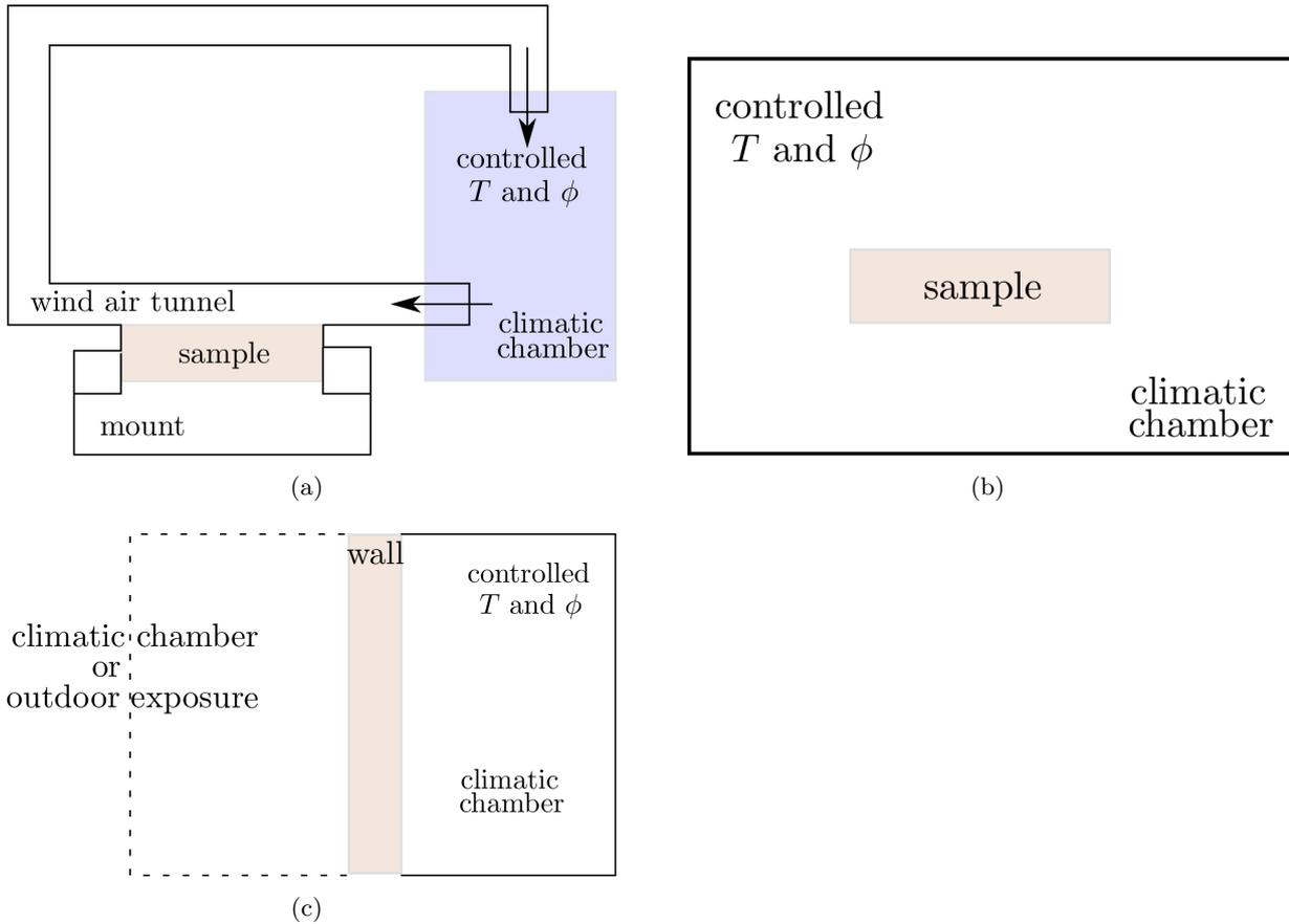
Figure 3: Experimental facility used to investigate the heat and moisture transfers: wind air tunnel (a), climatic chamber (b) and wall scale (c).
