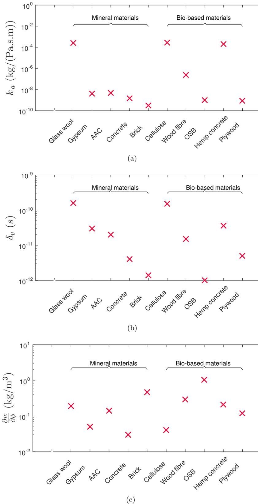
Figure 5: Air permeability (a), vapour permeability (b) and sorption capacity (c) of some materials used in the experimental investigations [104, 105]
