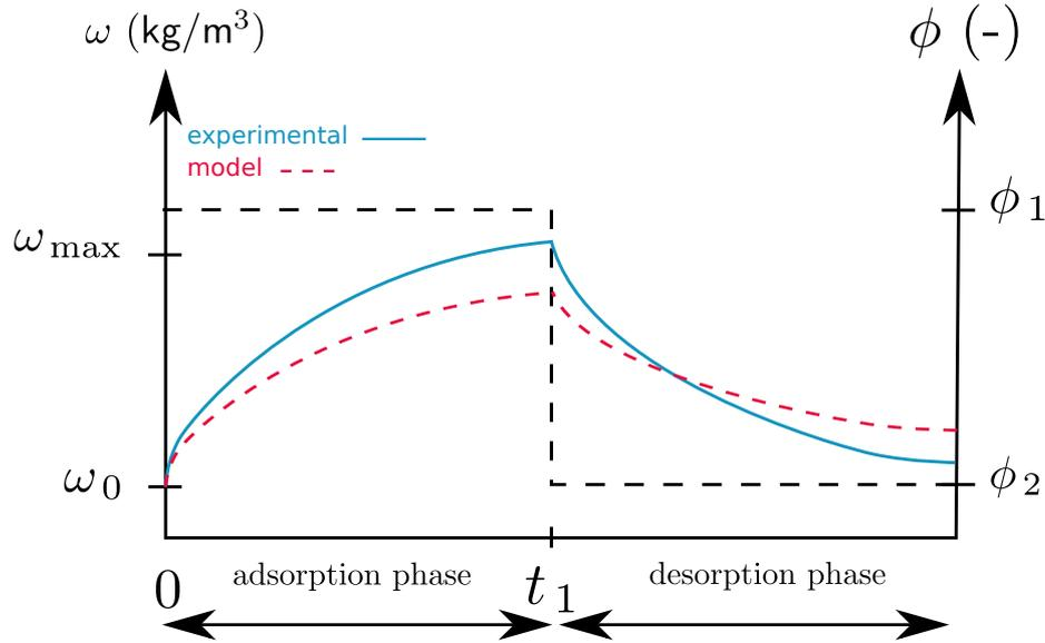
Figure 1: Illustration of the discrepancies when comparing experimental data and numerical results.
