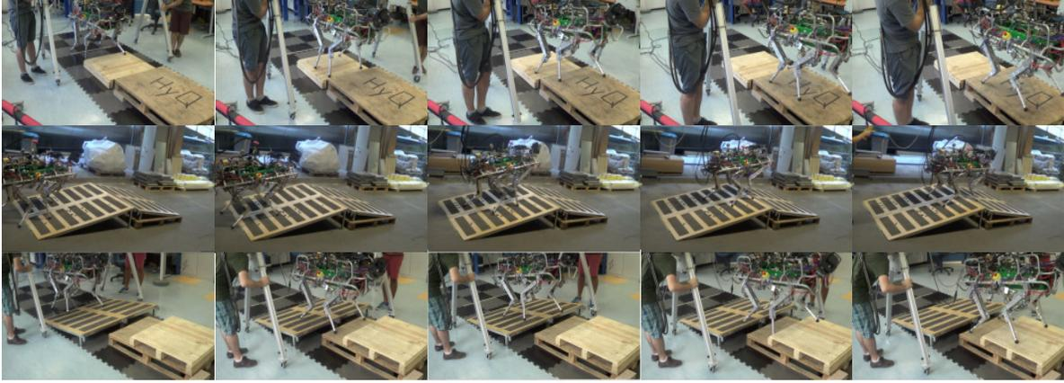
Fig. 8: Snapshots of experiments 1 through 3, used to evaluate the performance of our planner on challenging terrain. *Top*: Climbing a pallet and crossing a 20 cm gap, while climbing 3 cm. *Middle*: Climbing a  $10^\circ$  slope and crossing a 15 cm gap leading to a  $-10^\circ$  slope. *Bottom*: Climbing a  $10^\circ$  slope and crossing a 20 cm gap, while climbing down 6 cm leading to an 11 cm stair.
