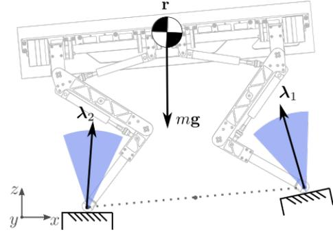
Fig. 3: Centroidal dynamic model of a quadruped.
