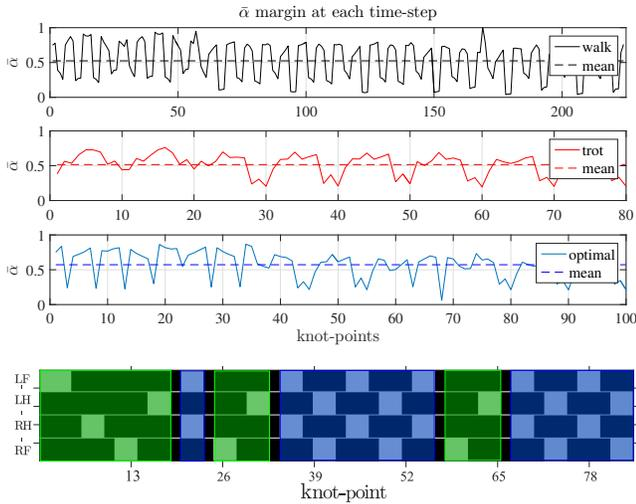
Fig. 11: *Top*: Normalized  $\alpha$  margin for different gaits. *Bottom*: Resulting optimal gait sequence for navigating in roof-like terrain, blue and green segments represent trot and walk, respectively.
