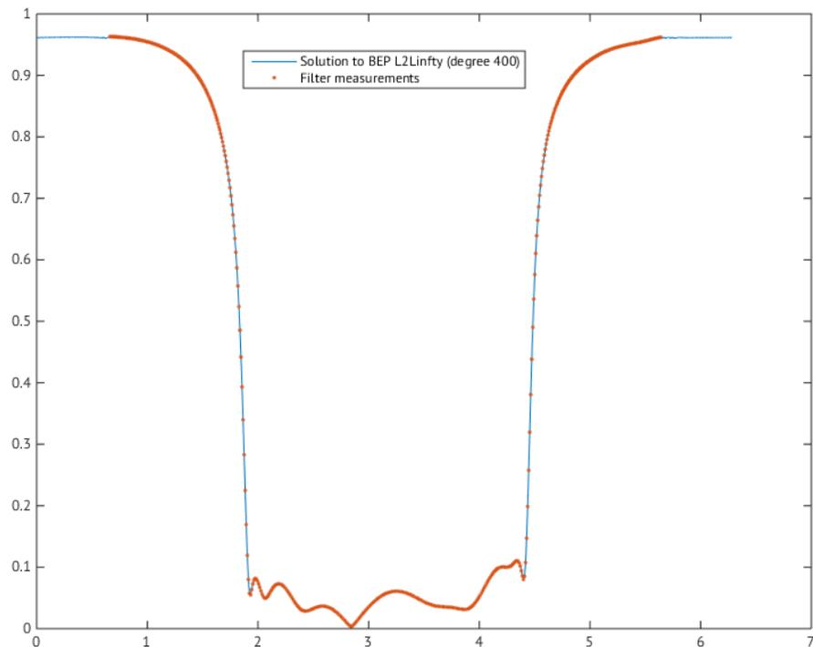
Figure 1: Solution of DBEP at hand of partial scattering measurements of a microwave filter
