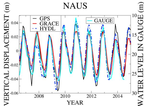
**Figure 2.** Vertical crustal displacement (cm) at NAUS station using different techniques, namely, the HYDL hydrological model, GRACE mission, and GPS positioning. Note that this station is at the same location in Manaus (cf. Figure 1), as the MANA station used by *Bevis et al.* [2005], now inactive.
