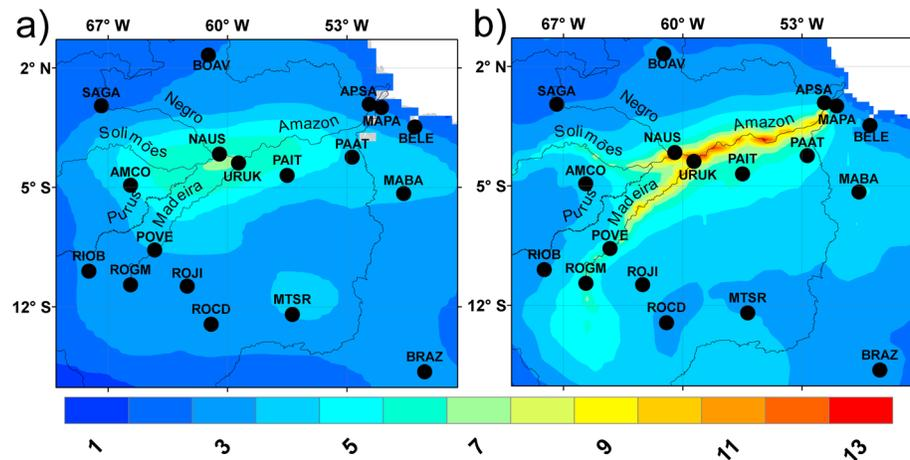
**Figure 1.** (a) GRACE-derived and (b) HYDL vertical displacement maximum amplitude (cm). Based on 2007–2014 GRACE (GRGS) and HYDL series. Black dots indicate the permanent GPS stations in the Amazon basin used in this study.
