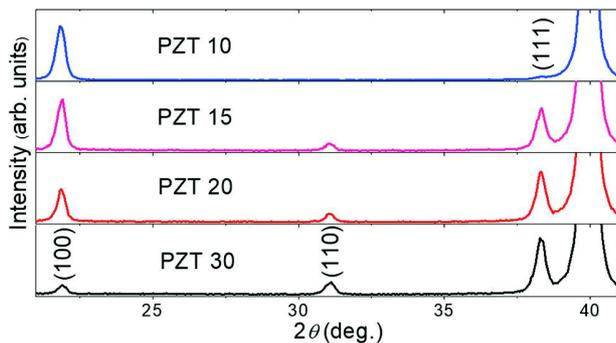
FIG. 3.  $\theta$ - $2\theta$  XRD scans for 10, 15, 20, and 30% Pb precursor excess.
