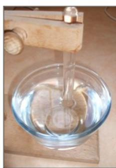
Torricelli's experiment is then presented, using water instead of mercury. The key Q1 is : “What happens if the tube filled with water is stood upside-down in a container of water?”
