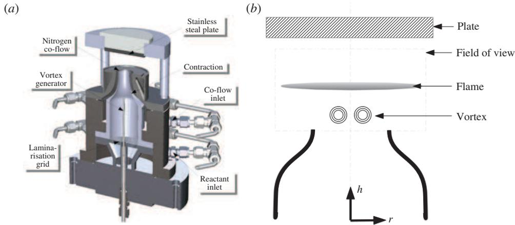
FIGURE 1. (Colour online) Schematic of the flame–vortex interaction burner (FVIB).
