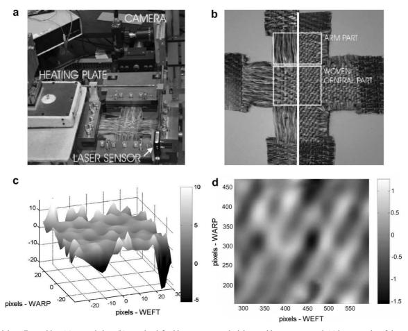
Fig. 6. Biaxial tensile machine: (a) general view; (b) samples, left: side yarns removed; right: no side yarns removed; (c) homogeneity of the tensile strains: first invariant field for test 1/1 with yarns removed; depicted is whole central area minus one yarn on the circumference; applied strain: 1.17% in weft, 2.23% in warp; (d) Shear angle field (degrees) for test 1/1 with yarns removed; depicted is the whole central area minus three weft yarn and five warp yarns on the circumference.
