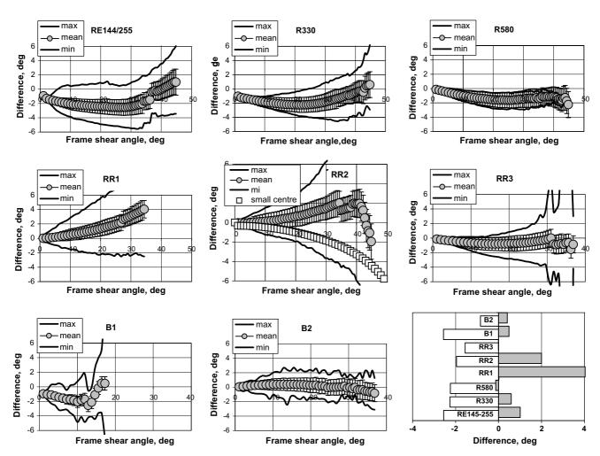
Fig. 3. Difference of the average shear angle of the fabric, measured using DIC, and shear angle of the frame. Graph for RR2: large and small sample configuration; other graphs: large sample configuration. Error bars indicate standard deviation in five tests. The last diagram: minimum and maximum differences for all the tested fabrics, large sample configuration.
