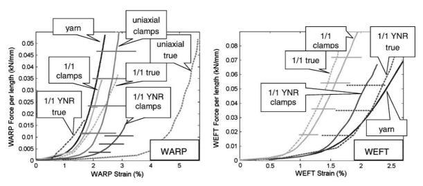
Fig. 7. Tensile diagrams in warp and weft direction, based on DIC-measured average sample strain ("true") and enforced strain ("clamps"), for samples with yarns removed (–) and not removed (YNR), together with tensile diagrams of the yarns.
