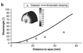
Fig. 10. Comparison of the measured shear angles and those obtained via a kinematical modelling approach for two blank-orientations: (a) 0°; (b) 45°. The "distance to the apex" indicates the distance along the arches shown in the insets.
