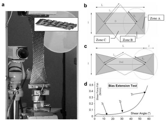
Fig. 4. Bias extension test: (a) the device (inset: weave structure of the fabric G1151); (b) initial rectangular specimen with yarns oriented at  $\pm 45^{\circ}$ ; (c) deformed specimen; (d) shear load curve for G1151 interlock fabric. Angles calculated from the mesoscopic analysis.
