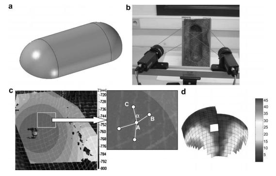
Fig. 9. Measurements of the local deformations of the shaped preform: (a) the mould; (b) set-up of LIMESS measuring system; (c) a correlated surface that depicts the *z*-coordinate of the surface in grey-scale overlaid on a picture of a deformed sheet; (d) calculated shear angle distribution.
