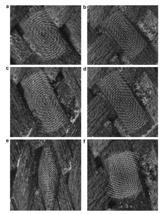
Fig. 8. Meso-scale analysis: displacement fields within a yarn. (a) Central zone C for d = 30 mm,  $\gamma = 22^{\circ}$ ; (b) zone B, d = 30 mm,  $\gamma^* = 8^{\circ}$ ; (c) central zone C for d = 50 mm,  $\gamma = 35^{\circ}$ ; (d) zone B, d = 50 mm,  $\gamma^* = 16^{\circ}$ ; (e) central zone C, d = 80 mm, C,  $\gamma = 56^{\circ}$ ; (f) zone B, d = 80 mm,  $\gamma^* = 39^{\circ}$ .
