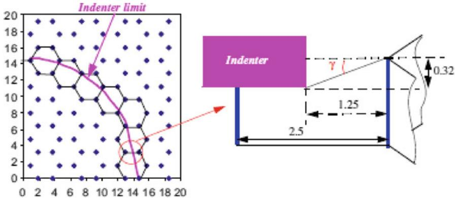
Fig. 28 Geometry for the computation of the limit  $\gamma$
