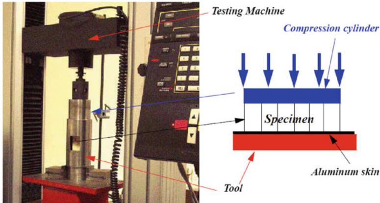
**Fig. 1** Test procedure for compression of honeycomb cores
