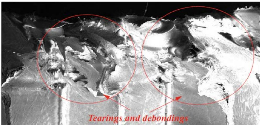
Fig. 6 Picture at point 11, damages in the honeycomb
