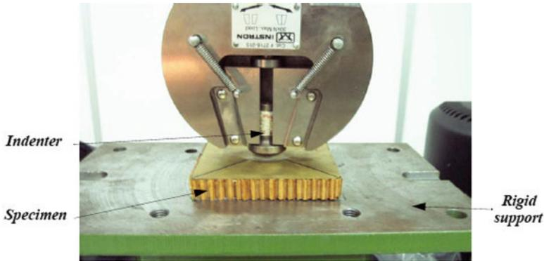
**Fig. 29** Description of the indentation tests on sandwich specimens
