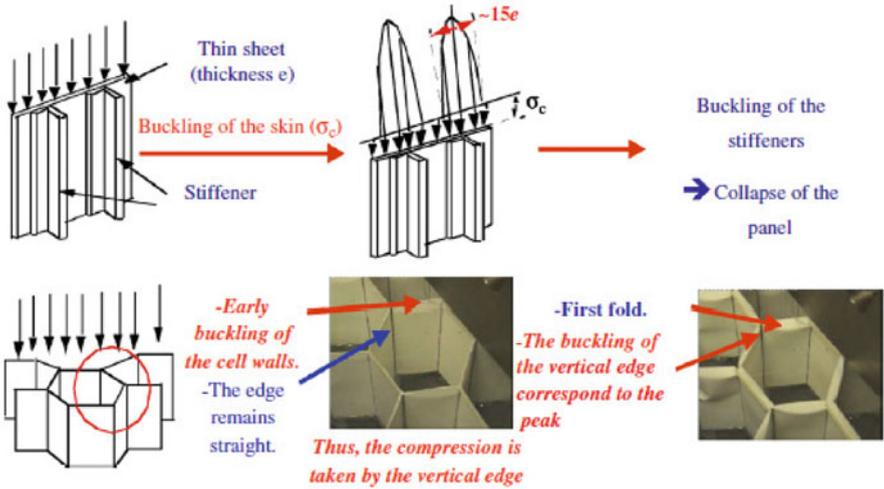
Fig. 17 Analogy with the buckling of stiffened panels
