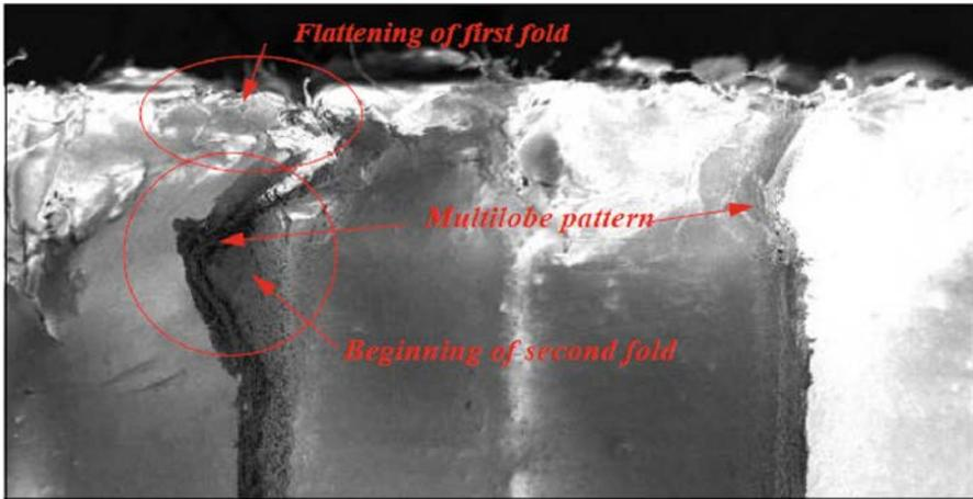
Fig. 5 Picture at point 8. Continuation of folding
