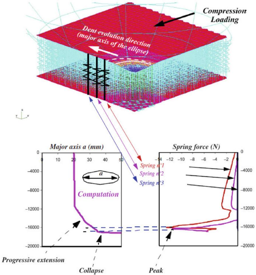
**Fig. 58** Analysis of the collapse of pristine core after impact
