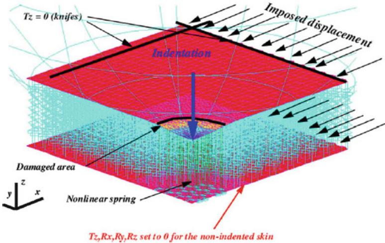
Fig. 52 Finite element model for compression after impact
