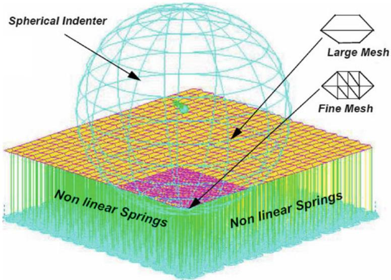
Fig. 35 Finite element modeling of the indentation problem on sandwich with thin metal skins
