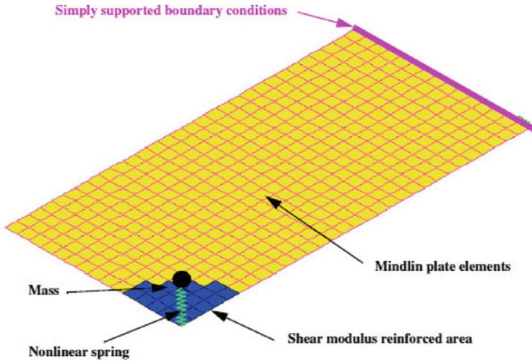
Fig. 43 Spring-mass finite element model
