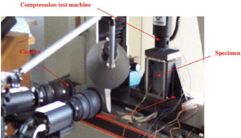
Fig. 46 CAI test device
