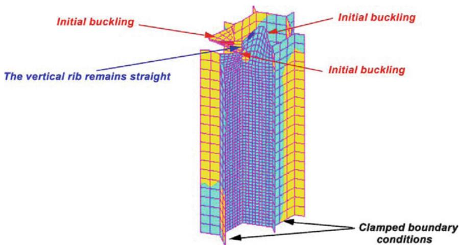
**Fig. 16** Initial buckling mode of a Nomex hexagonal cell under uniform compression
