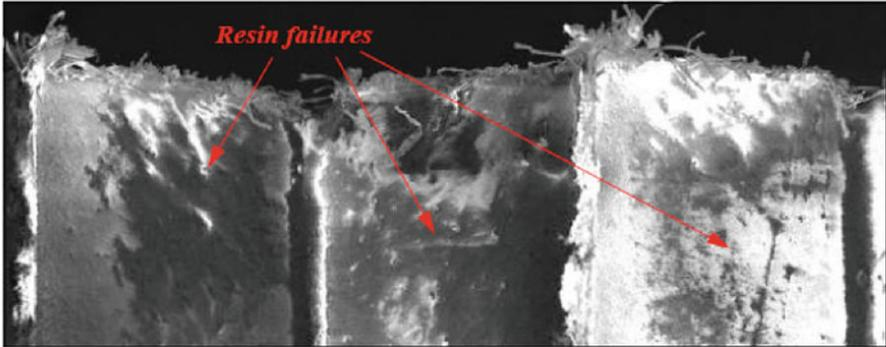
Fig. 3 Picture at point 2, view of resin failures
