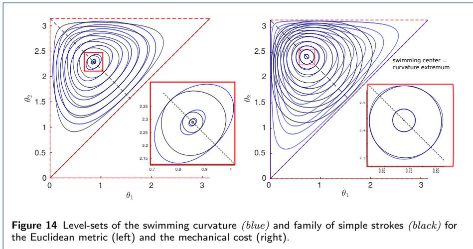
**Figure 14** Level-sets of the swimming curvature (blue) and family of simple strokes (black) for the Euclidean metric (left) and the mechanical cost (right).
