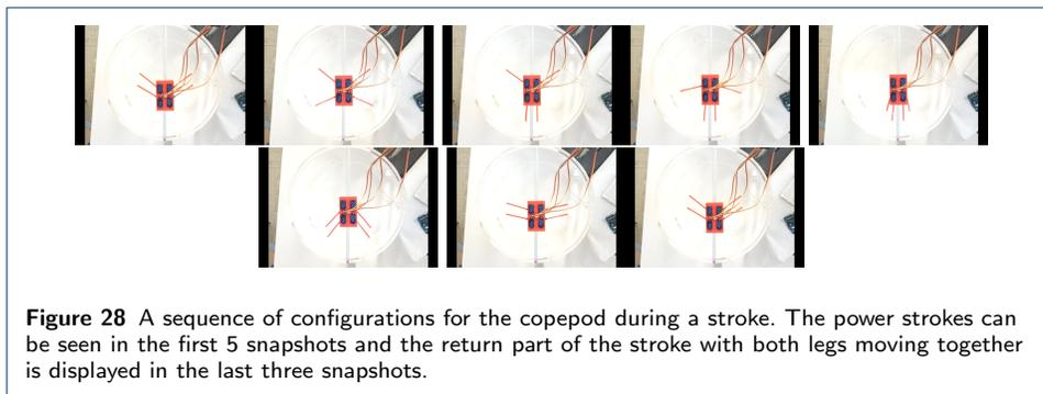
**Figure 28** A sequence of configurations for the copepod during a stroke. The power strokes can be seen in the first 5 snapshots and the return part of the stroke with both legs moving together is displayed in the last three snapshots.
