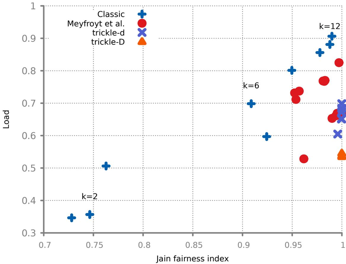
Figure 12: Fairness and load results for Trickle tests on three IoT-lab platforms with 15, 30 and 50 nodes. "Classic" shows several  $k$  values; "Meyfroyt" several  $\alpha$  values; "Trickle-d" several parameter sets and "Trickle-D".
