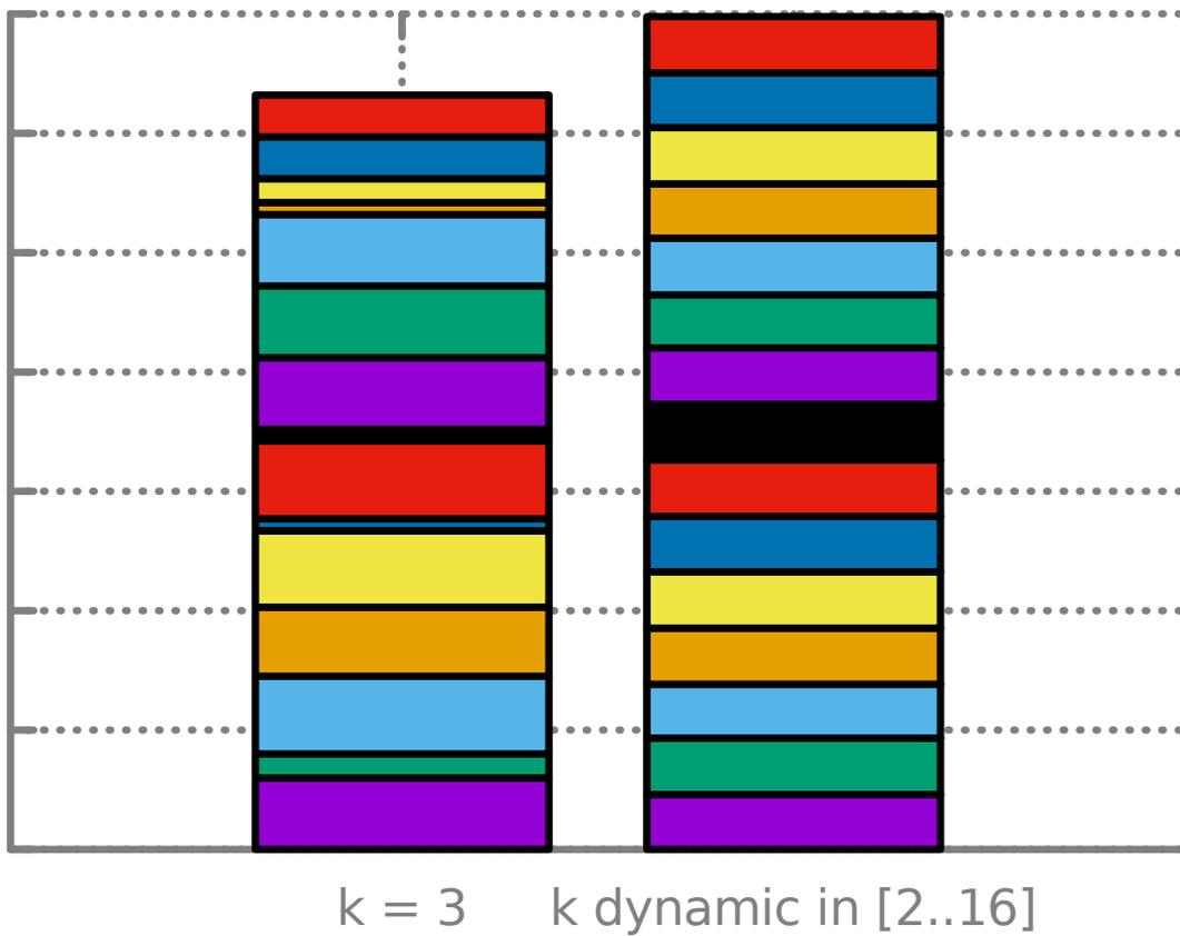
Figure 8: Typical message count per nodes repartition for  $k = 3$  and  $k$  dynamically adjusted. Each node is represented by a color and the rectangle surface is proportional to its transmission load.
