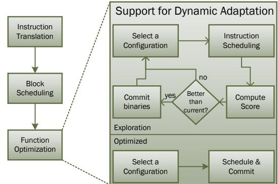
Fig. 3. Details on the flow handling dynamic adaptation
