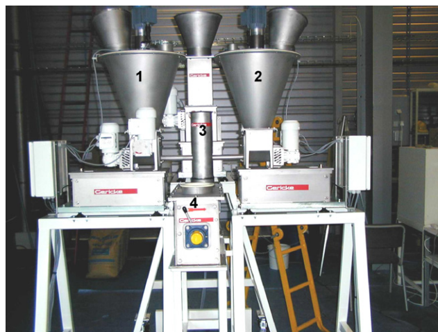
Fig. 1 – Pilot-scale continuous mixer: loss-in-weight feeders (1 and 2), feeding chute tube (3), and mixer (4).
