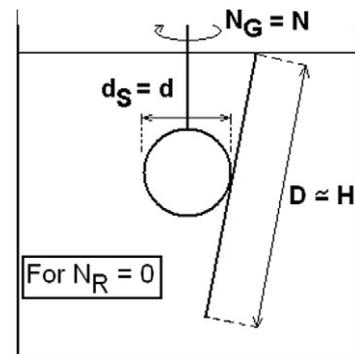
Fig. 3. Analogies between the geometric parameters of the classical mixing system and the TRIAXE<sup>®</sup> planetary mixer when rotational speed is set to zero.
