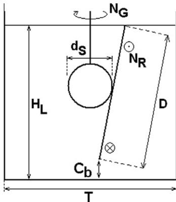
Fig. 2. Sketch and symbols used for the TRIAXE<sup>®</sup> system investigated.
