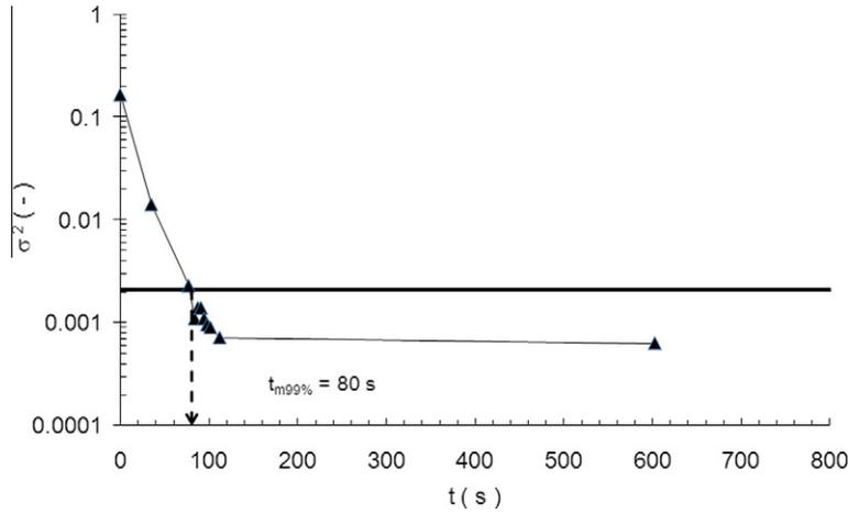
Fig. 8. Determination of mixing time  $t_m$ .
