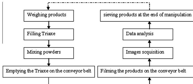
**Fig. 7.** Diagram of the experimental protocol.
