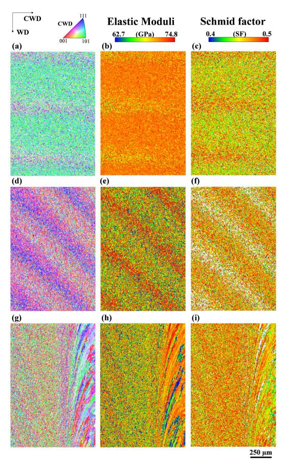
Fig. 13. EBSD maps of the different reference regions to the macroscopic loading direction (CWD) of the shoulder-affected region in the CWD-WD plane located 150  $\mu$ m beneath the top surface: (a, d, g) IPF, (b, e, h) Elastic moduli, (c, f, i) Schmid factor (White grains correspond to grains having a Schmid factor below 0.4). (a, b, c) AS + 1 mm region, (d, e, f) AS + 5 mm region, (g, h, i) AS + 7 mm region.
