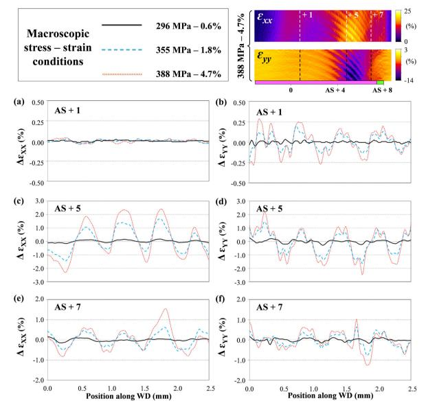
Fig. 11.  $\Delta$ ε<sub>XX</sub> and  $\Delta$ ε<sub>YY</sub> profiles along WD at different locations within the nugget showing the difference in HDB/LDB pattern extension. The positions of the  $\Delta$ ε<sub>XX</sub> and  $\Delta$ ε<sub>YY</sub> profiles are depicted as dashed lines in the top right insert. a) and b) AS + 1 mm, c) and d) AS + 5 mm and e) and f) AS + 7 mm.
