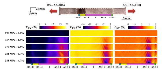
Fig. 9. Local in-plane strain distribution obtained with DIC corresponding to various macroscopic strains (based on a 30 mm gage length) and represented in three columns. The top incrustation illustrates the area of interest of the joint used for DIC measurements.
