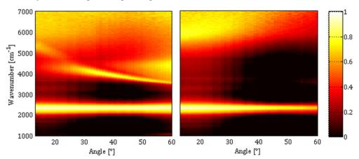
Fig. 5. MIMs emissivity characterization in TM (left) and TE (right) polarization using a polarizer on the optical path of the FTIR.
