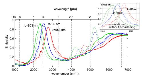
Fig. 3. Measured and simulated MIM spectral emissivities from the reflectivity spectrum at 13° from normal incidence, for three different sizes L of patches as indicated. Solid lines: experimental; dashed lines: simulation with empirical Lorentizan-type broadening included; inset: peak region with non-broadened RCWA simulations (dashed lines).
