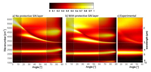
Fig. 2. (a) Emissivity simulation of L=803 nm MIM resonators as those of Fig. 1(a), and colorbar on top; (b) same simulation with an extra SiN 100-nm-thick added protective layer; inducing a red shift of the resonance; (c) characterization of realized MIMs. The angular range of this characterization is the one not shaded in (a,b). Simulations are carried out with RCWA, while characterizations rely on a setup involving an angularly resolved FTIR.
