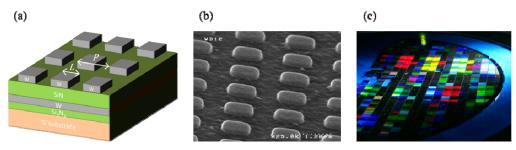
Fig. 1. (a) Illustration of the MIM structure; (b) Scanning Electron Microscope (SEM) image of the realized resonators; (c) 200 mm silicon wafer with MIMs. Each die is  $5 \times 5 \text{mm}^2$  and consists of a specific kind of MIMs.
