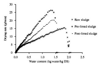
$\textbf{Fig. 15.} \ \ \textbf{Influence of liming on the evaporation flux during convective drying [42]}.$
