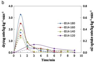
**Fig. 23.** Influence of the oil temperature on the sludge drying behavior during frying [55]. (a) Variation of the product moisture content and its temperature, (b) drying rate.
