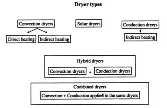
Fig. 1. Types of dryers used for sludge wastewater drying [2].
