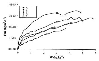
**Fig. 7.** Influence of the origin of sludge on its behavior during convective drying [6]. (A) and (B) Domestic sludge with respectively 8000 and 9000 population equivalents, (C) agro-food industrial sludge, (D) domestic sludge with 27,000 population equivalents, (E) mixture between agro-food industrial sludge and domestic sludge.
