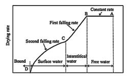
Fig. 5. Typical wastewater sludge drying curve [1].
