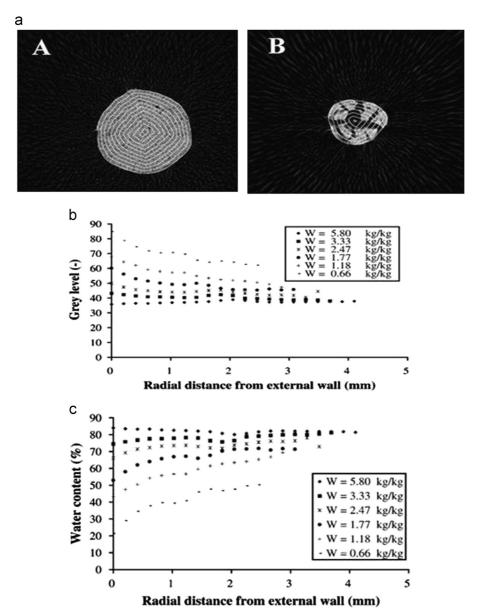
Fig. 13. Grey level measurement [37]. (a) Grey level measurement, (b) grey level profiles at the different water contents, (c) distribution of the moisture profile.
