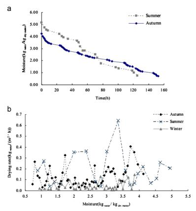
Fig. 22. Evolution of the drying rate during solar drying [52]. (a) Moisture content, (b) drying rate.
