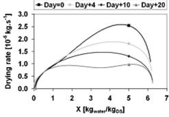
Fig. 17. Influence of the storage during on the drying kinetic behavior of wastewater sludge [43].
