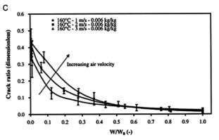
**Fig. 12.** Influence of the sludge origin and operating conditions on shrinkage and cracks extent. (a) Shrinkage [36], (b) cracks [36], (c) effect of the air velocity on cracks.
