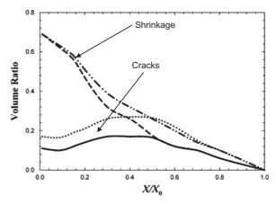
Fig. 9. Variation of shrinkage and cracks during convective drying of wastewater sludge [12].
