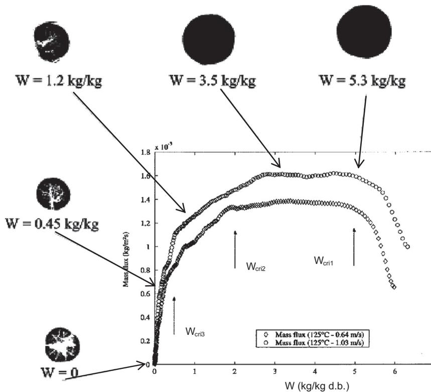
Fig. 11. Shrinkage and cracks formation during convective drying [36].
