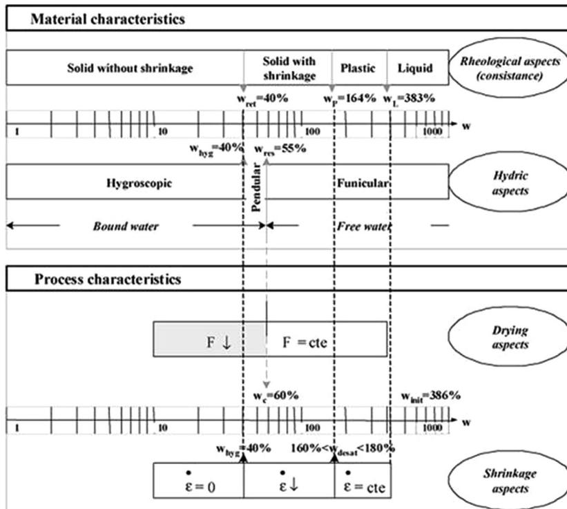
Fig. 14. Hydric and rheological aspects during convective drying [28].
