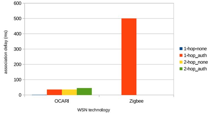
**Fig. 7.** Association delays comparison with and without authentication
